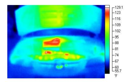
Since the cp- $e^{TM}$  intercooler is in front of the car, it will receive very little heat transfer. This is ideal as the intercooler is now only responsible for cooling the intake air, as opposed to waste heat from the engine. You can see the blue rectangle behind the bumper, which indicates a temperature of about 75°F.
