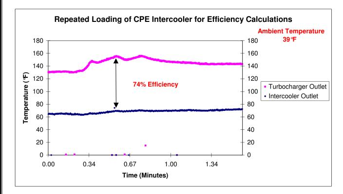
Compare the stock intercooler's efficiency to the cp-e<sup>TM</sup> intercooler:
