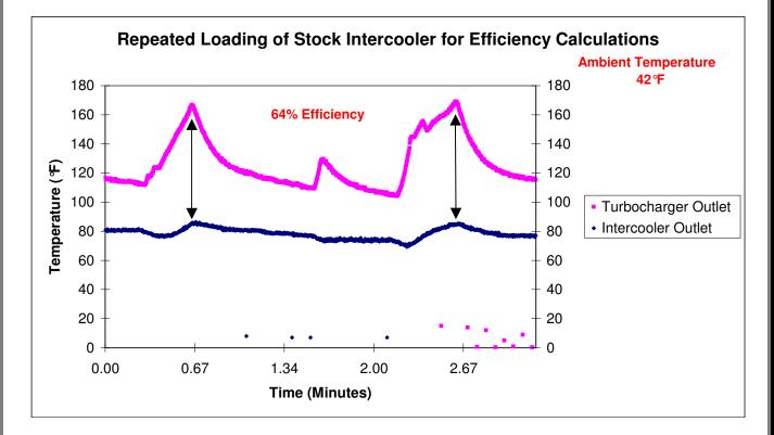
But using these calculations are not as straightforward as one might think. A well-known tactic in drag racing is to "ice down" the intercooler before a race. This artificially raises the intercooler efficiency since it will drop the core temperature below ambient. So, the temperature of the core is also of great significance, as it will affect the efficiency calculations. So, we opted to perform several runs to illustrate this point, and to show how sensitive the stock core is to temperature.
