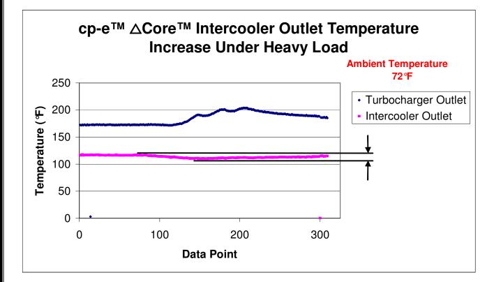
Notice the temperature increase of both the boosted air before and after the intercooler. Despite a  $40^{\circ}$ F increase in boosted air temperature, the temperature of the air exiting the cp-e<sup>TM</sup> intercooler is almost unchanged! In fact, the intercooler outlet temperature seems to *drop* once the throttle is pinned. This is probably due to the increase in air speed while the throttle was applied.
