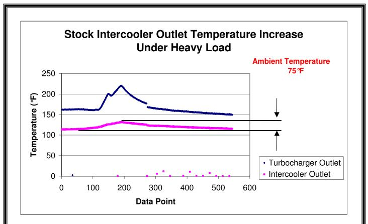
Notice how sharply the temperature of the air coming out of the intercooler increases under boost. Even though the boosted air is hotter than the  $cp-e^{TM}$  example, the stock intercooler increases the outlet temperature by as much as 30°F! If we had been able to load the intercooler for longer than a few seconds, the problem would be even more apparent.
